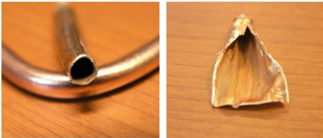
Figure 11. Grooved Wick Type Heat Pipe
